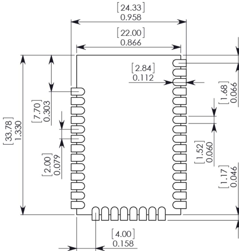
***XBee3 Micro recommended footprint***
