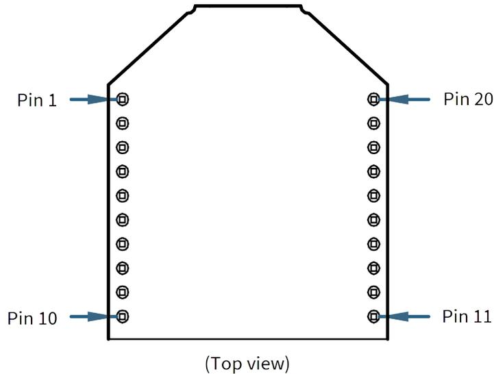
The following table shows the pin signals and their descriptions for the XBee3 through-hole device.
